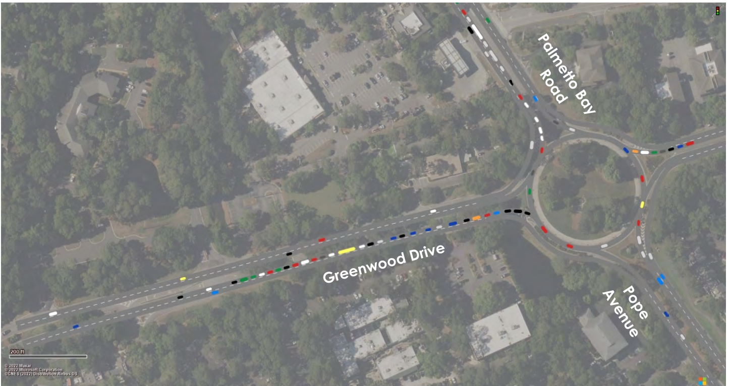
FIGURE 49: EASTBOUND GREENWOOD DRIVE APPROACH QUEUE AT SEA PINES CIRCLE – 2023 NO-BUILD AM
