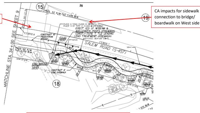
Proposed Design from Plans for East Side at Bridge CA = Critical Area Delineation
